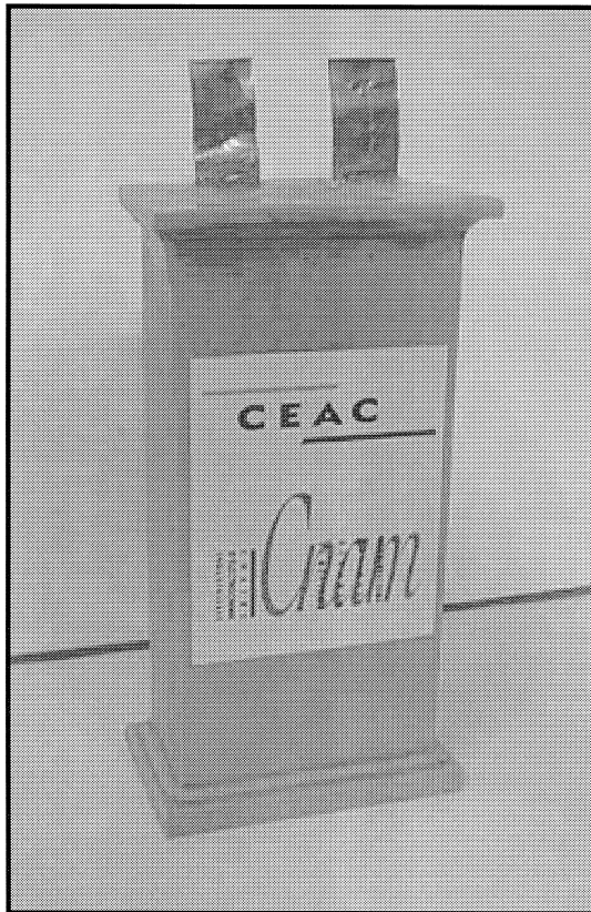
Fig. 8. Supercapacitor SC#3. Weight of the supercapacitor: 134 g, volume: 100 cm 3 .
